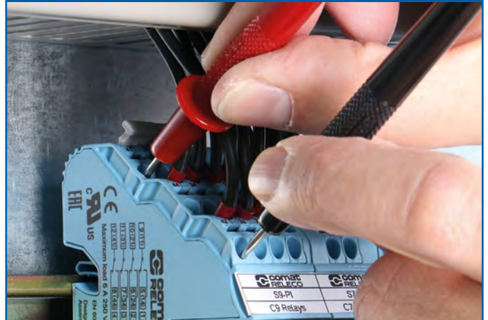
Application of test probes in contact terminals
