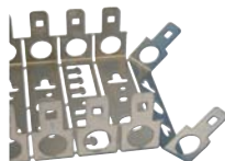
LSA 2/10-MW10-25/22 (Art.-No. 24 01 10) LSA backmount frame 10 x 10DA (modular) stainless metal. Plug space for 10 pcs of LSA 2/10 10DA connection modules (Σ 100 DA) 25 mm grid / depth 22 mm, easily detachable upon individual requirements, available up to a size of 78 connection modules.
