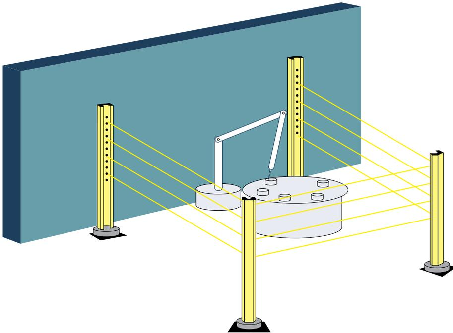
In applications where the monitoring of an area is required, safety light curtains can be used together with mirror for perimetral protection.
