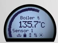
Through the glass, you can easily monitor the process value, and the radial bar graph indicates the process magnitude at a glance. A custom device tag, process value tag and unit fields make it easy to identify the displayed process point.
