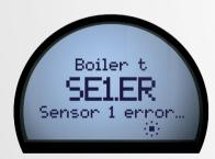
If a sensor or device error occurs, a red or white flashing backlight, specific error text, and scrolling error messages help you provide quick troubleshooting.
